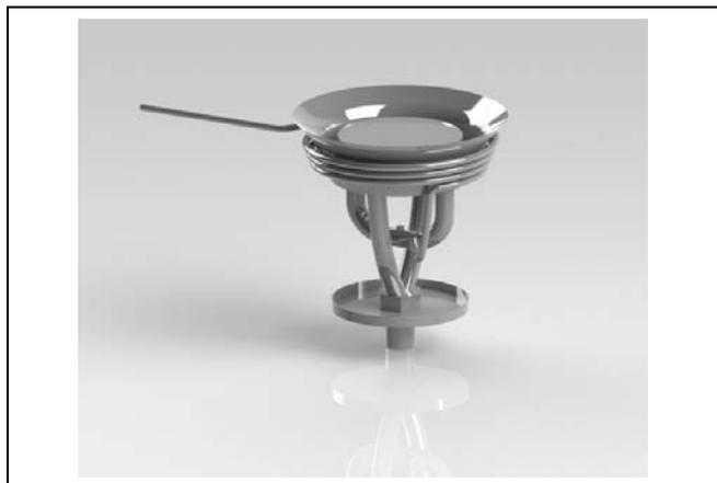
Fig 4: Burner Assembly of Vapor Jet Stove
